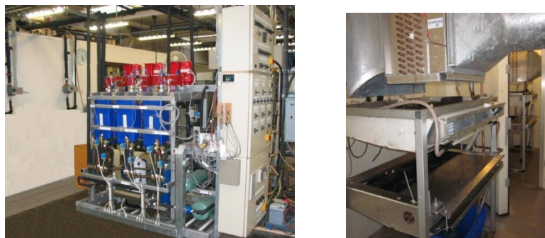
Figure 3 (b)/(c). Transport Refrigeration Test Rig: (a) Primary system with twin insulated compartments to rear. (b) Inside insulated compartments with associated DX evaporators (middle) and IDX remote coolers (top/bottom).
