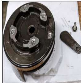
Discharge side with the check valve removed
